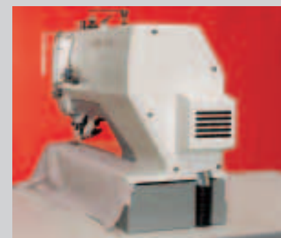
Servo sewing drive integrated in housing
