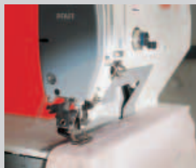
Off-set arm for easy placing/handling of workpiece
